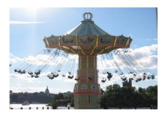
The swings hang out because a sideways force from the chain is needed to change the motion - otherwise the swings would just continue forward in a straight line.
