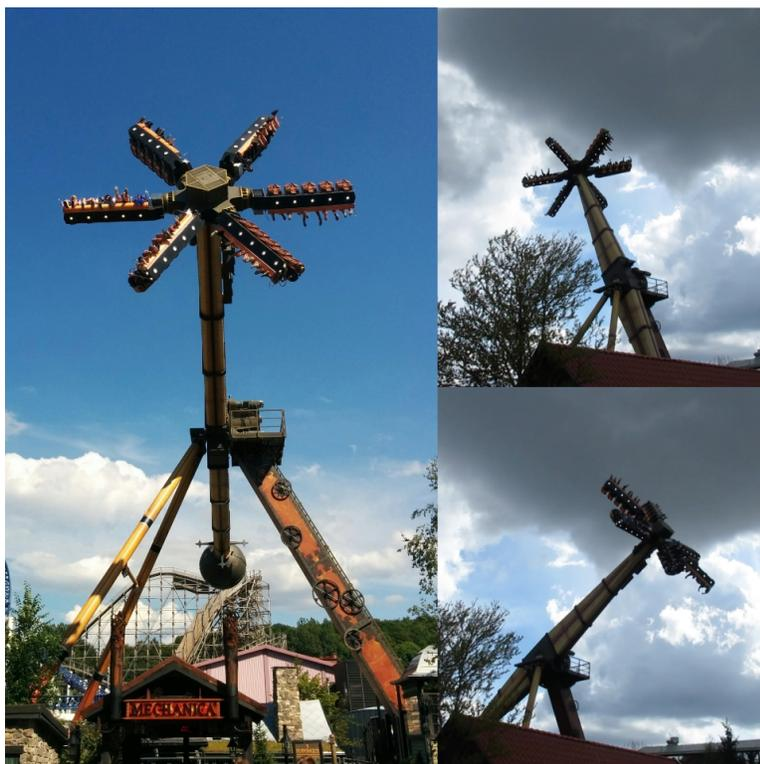
**Figure 1.** The Star Shape ride Mechanica at Liseberg. The 12 m main arm rotates a full turn in 8 s. At the same time the star, with a radius of 4 m, rotates a full turn in 10 s. Each of the gondolas in the star seats 5 guests, and can rotate freely around its axis, as discussed in more detail in section 3.
