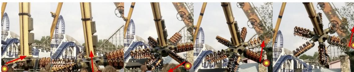
**Figure 6.** The motion of a rider passing the lowest point of the ride, while rotating around the arm of the star. The arrows mark the "up" direction for the rider and the time interval between the screen shots is 0.4s.
