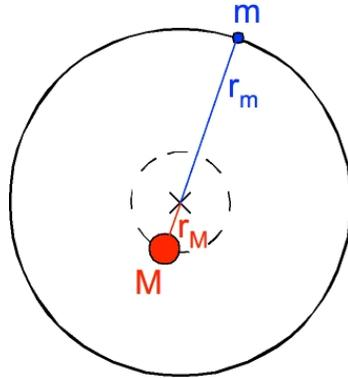
**Figure 2.** Illustrations of "planetary orbits" of an object with mass  $m$ , around a heavier body with mass  $M$ . Their distances to the centre of mass are related as  $r_M = r_m(m/M)$ .
