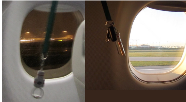
Fig. 1 A keyring hanging from a string during takeoff and landing of an airplane (previously published [1].)
